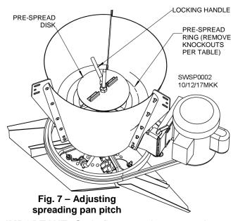
**IMPORTANT:** Grain flow must be centered over pre-spread disc for even spreading.
