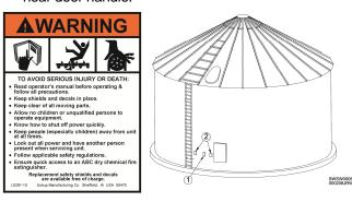
2. **DECAL L0258A – DANGER:** Do not enter this bin! **Mount this decal** on bin sheet near door handle and at all other entry points. Also mount this decal at eye level on bin sheet near ladder going to roof.
