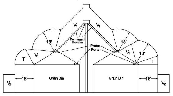
V<sub>1</sub> = Vertical clearance above a building required by Rule 234C (Table 234-1)
