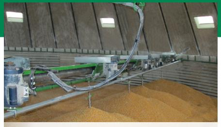
With a patented mechanical reversing drive, the Sukup Fastir® makes other stirring machines with cable or chain drives obsolete.
